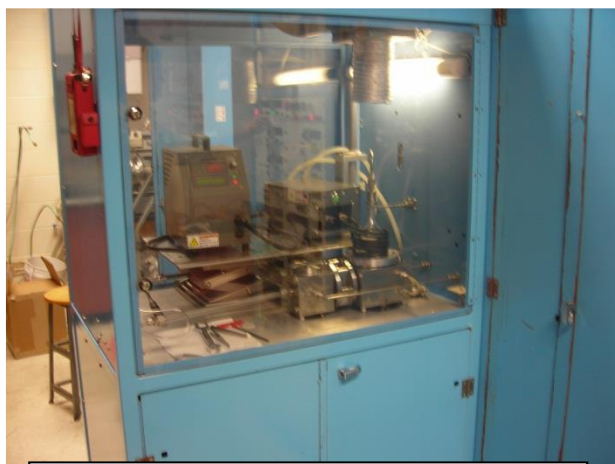
Image 5: MOCVD System with MOCVD chamber pictured in center
