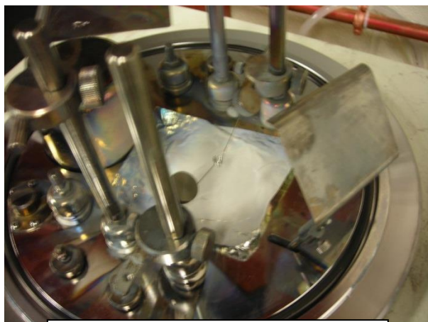
Image 1: wire basket in vacuum evaporator
